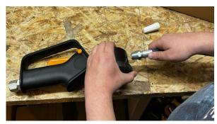
2. Start to tighten the hose manually.
