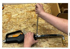
3. Finish tightening it using the wrench (23 mm)
