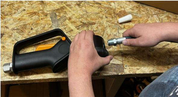
2. Start to tighten the hose manually.
