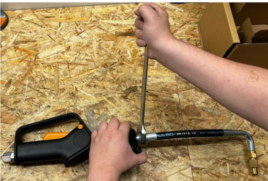
3. Finish tightening it using the wrench (23 mm)
